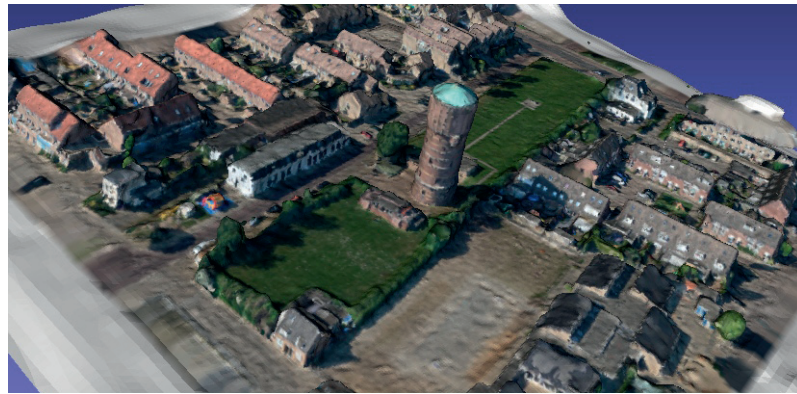
▲ Figure 4, Dense matching result (PMVS2: patch-based multi-view stereo software) and meshing (Meshlab, Poission reconstruction).
